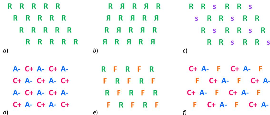
Schematic bidimensional representation of the structure of: (a) and (b) two polymorphs of a mono-component crystal; (c) a solvate; (d) a salt; (e) a cocrystal; and (f) a cocrystal of salt. (R: drug molecule, s: solvent molecule, A-: anionic moiety, C+: cationic moiety, F: neutral coformer molecule)
