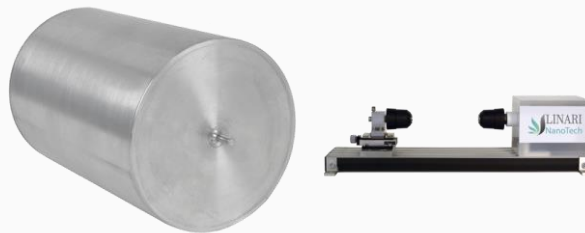
Figure 2: Linari stainless steel rotating drum collector and digitally controlled rotation system
