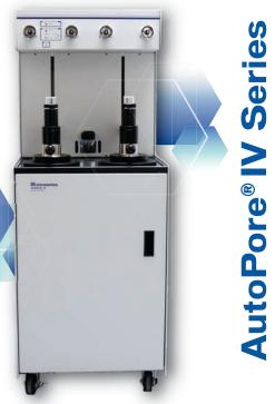
The AutoPore IV series uses mercury intrusion and extrusion to determine total pore volume, pore size distribution, percent porosity, density, compaction/compression and fluid transport properties.
