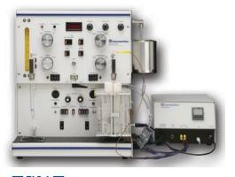
**ChemiSorb 2720** – Dual station, one for analysis and one for sample preparation
