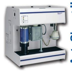
**The AutoChem II** performs a full array of highly precise, temperature-programmed studies. It uses the dynamic (flowing gas) technique to perform pulse chemisorption and temperature-programmed methods – reduction (TPR), desorption (TPD), oxidation (TPO), and reactions (TPSR) – as well as BET surface area evaluation.
