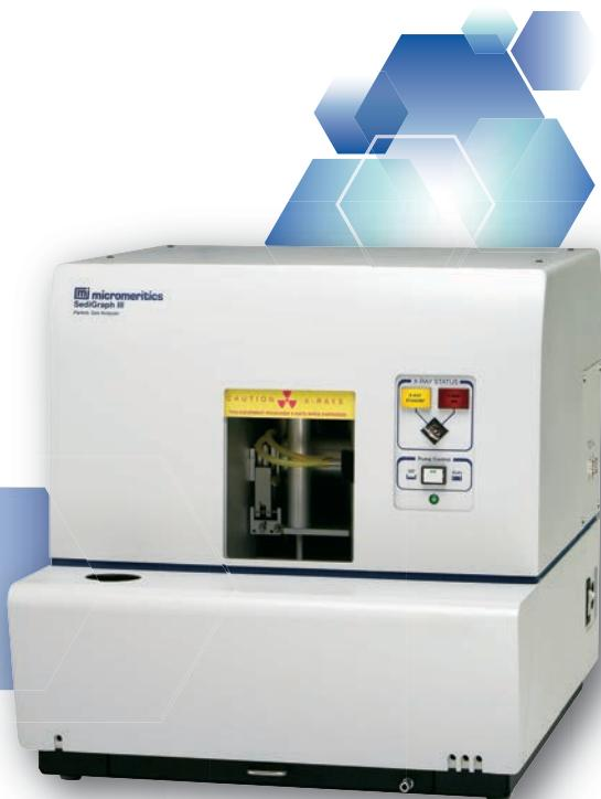
The SediGraph III analyzer combines the proven SediGraph analytical technique with advanced instrumentation features to provide superior repeatability, accuracy, and reproducibility. The SediGraph III uses x-ray absorption to measure mass concentration and Stokes' Law to determine particle size.
