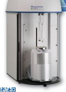
The TriStar II is an automated, three-station, surface area and porosity analyzer capable of increasing the speed of quality control analyses with the accuracy, resolution, and data reduction features to meet most research requirements.
