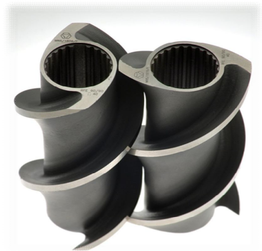
Figure 3. Shovel Elements for overcoming feed limitation
